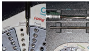
A Fixing Screw with 5mm in length was connected to Fixing Screw Driver coupled to Driver Handle.
