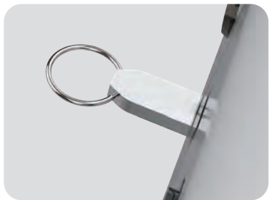
*USB Device to upgrade software or store data
